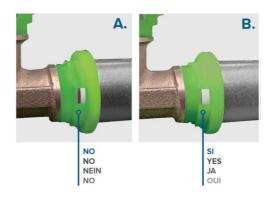
The picture "A" shows a non-correct introduction of the pipe into the fitting. The picture "B" shows a correct introduction of the pipe that is correspondence of the head of the plastic ring.
